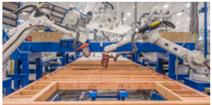
Above: Prefab Logic digital twins contain all building data and make building components easy to view. Autovol robots do the heavy lifting so tradespeople can work smarter.
